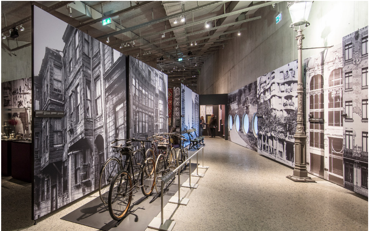
Hanging tension frames carrying double-sided textile prints for an exhibition at the National Museum in Zurich.
